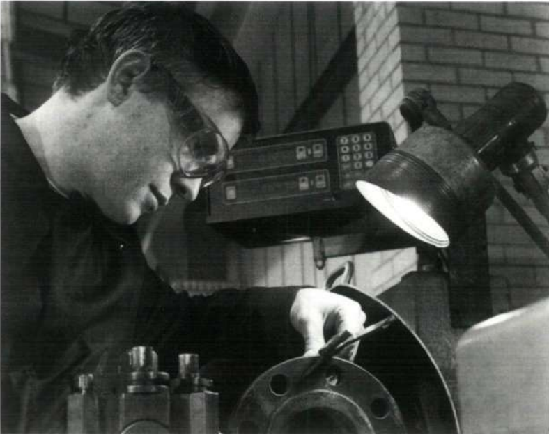
Figure 9 Local lighting providing flexible, directional lighting
