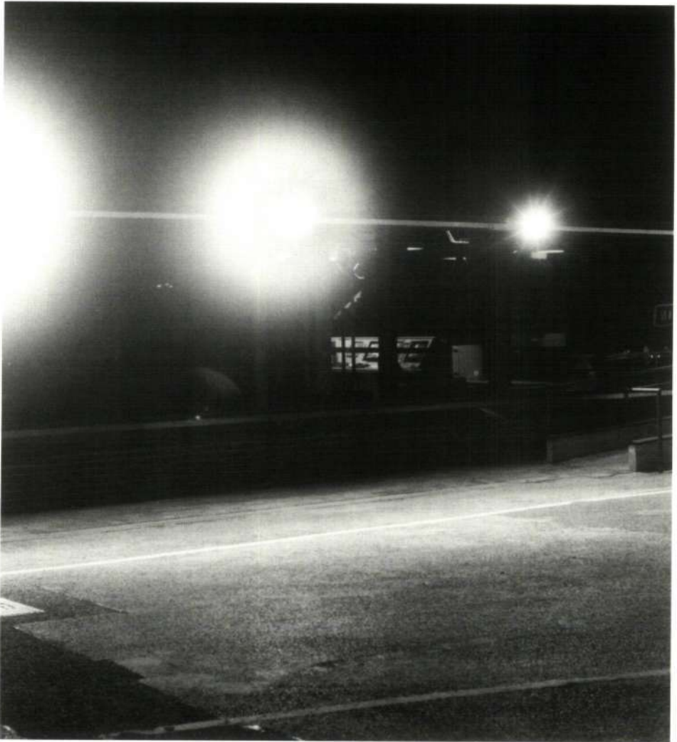
Figure 1 Disability glare from a light fitting
