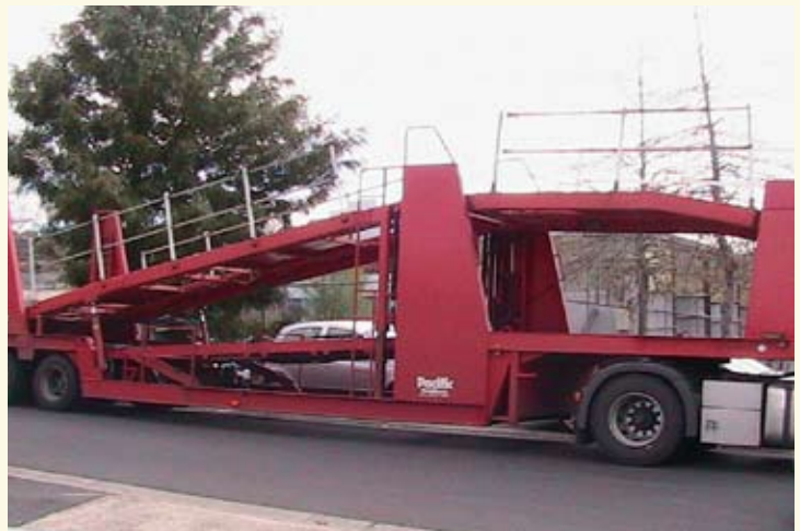
Car-carrier with fall protection railings
