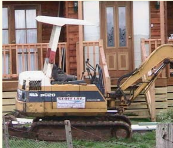
Tilt-down roll over protection on a small earthmover. Photo: J.Culvenor
